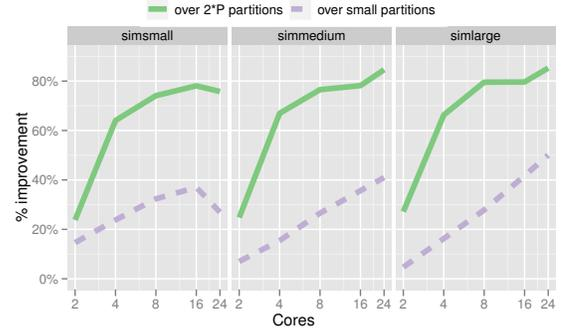
Fig. 14. Summary of improvement of dynamic partition refinement over static partitioning.
