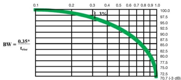
Figure 1. Oscilloscope Bandwidth vs. Frequency.
