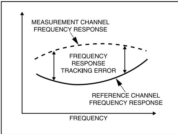
Figure 2: Response Tracking Error.
