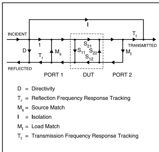
Figure 7: Forward Two-Port Error Model.
