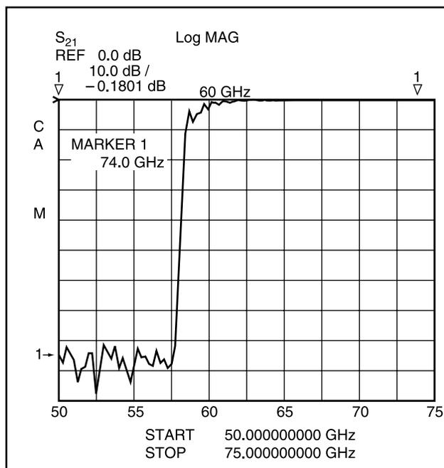
Figure 17: High Pass Filter Measurement.
