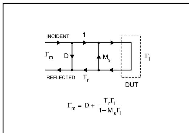
Figure 8: Error Model Modification for One-Port Measurements.
