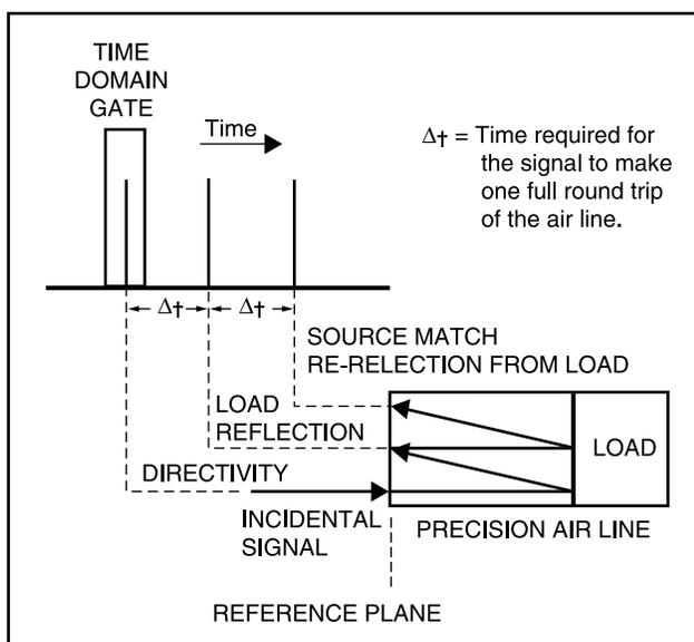
Figure 9: Time Domain Gate Isolation of Effective Directivity.
