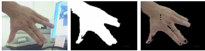
Figure 3. The image on left is colour-segmented to find the skin-colour pixels (middle). The two images are then combined to produce the VideoArms image on the right.
