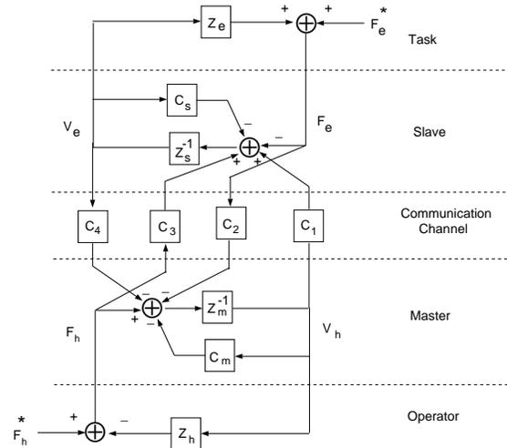
**Fig. 2 General teleoperator structure: After Lawrence, 1992**
