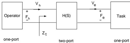
**Fig. 1 Network representation of teleoperator system**
