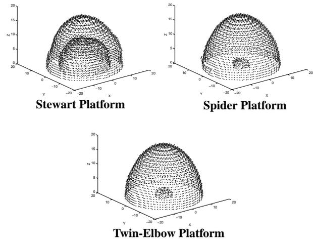
**Figure 10: Example Workspaces of Candidate Robots**
