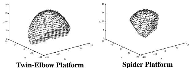
**Figure 11: Example Workspaces with U-Joint Constraint**
