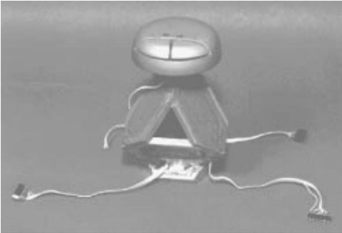
Figure 2: Maglev joystick flotor
