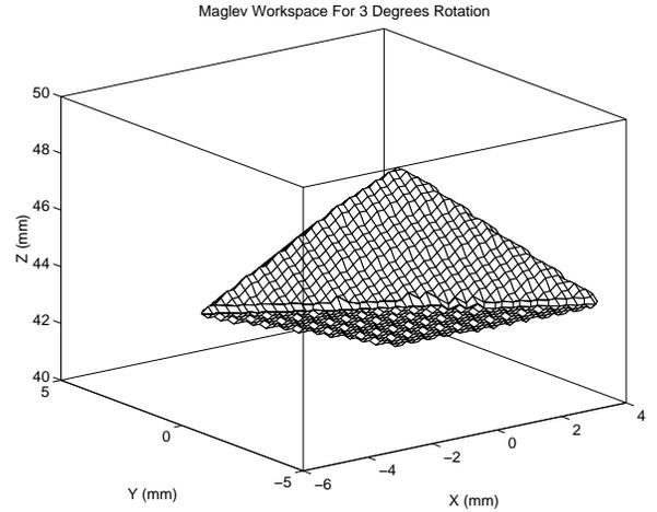
Figure 11: Optical sensor translational workspace for arbitrary rotations not exceeding  $3^\circ$ : the  $z$ -axis is the height of the vertex with respect to the PSD plane  $\pi$
