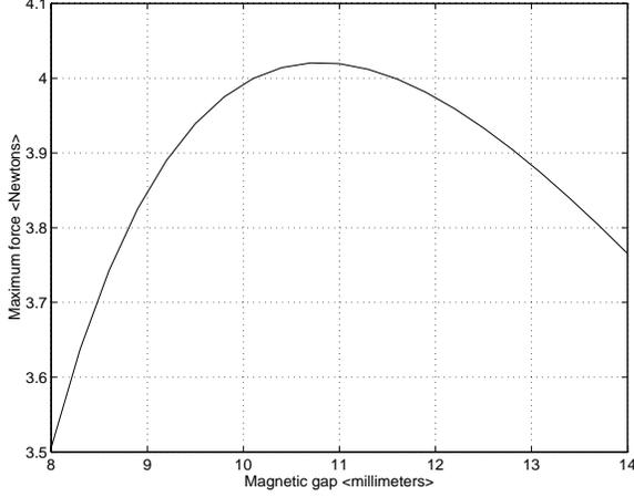
Figure 7: Actuator force vs gap with  $d_r = 6\text{mm}$  at  $P_{coil} = 8\text{W}$  ( $l_m = 20\text{mm}$ ,  $w_m = 8\text{mm}$ , and  $t_m = 4\text{mm}$ ), giving actuator gain at a current of 1A.
