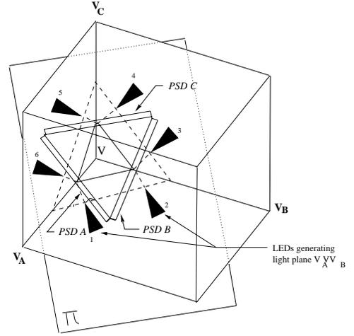
Figure 10: LED configuration for optical sensor
