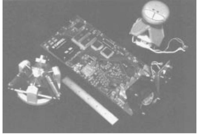
Figure 3: Maglev joystick stator, flotor and controller board.
