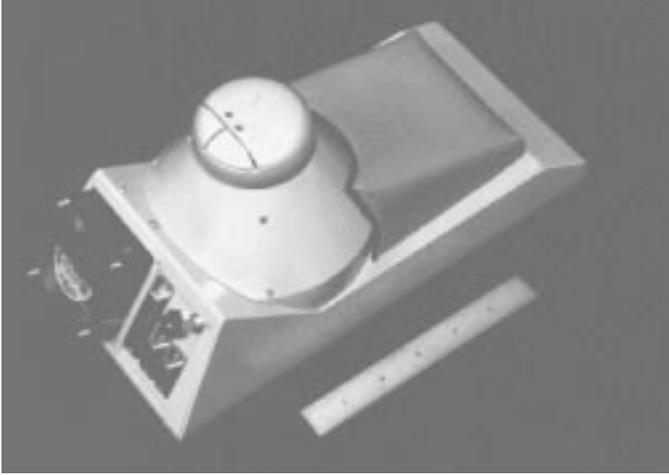
Figure 1: Photograph of the maglev desk-top joystick: a sloped support allows the user to easily grasp the disk-shaped handle.
