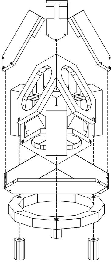
Figure 4: Haptic Interface Assembly Schematic
