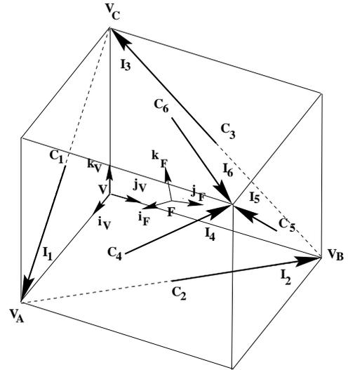
Figure 6: Coordinate assignments, coil centers and current vectors.
