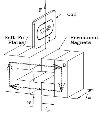
Figure 5: Basic Flat Coil Actuator
