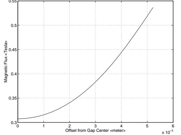
Figure 8: Predicted gap field at optimum gap (11mm)
