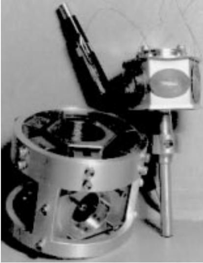
Figure 5: Micro-wrist stator and flotor
