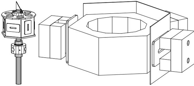
Figure 6: Flotor and Actuator Configuration
