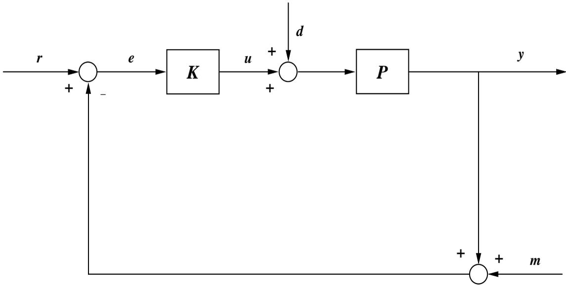
Figure 1: The closed-loop system.
