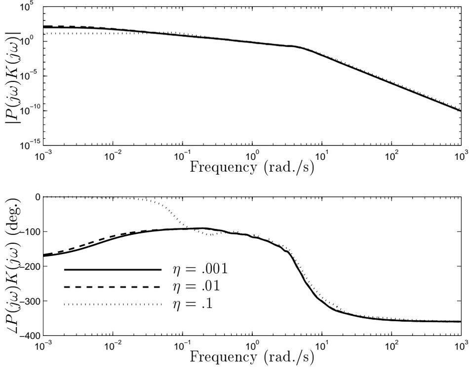
Figure 5: (a) and (b) show the Bode magnitude and phase plots respectively of the open-loop gain for the tuned system. The gain margin is approximately 15 dB for all three noise levels meeting the design specification. The phase margin is approximately 72 degrees for all three designs.
