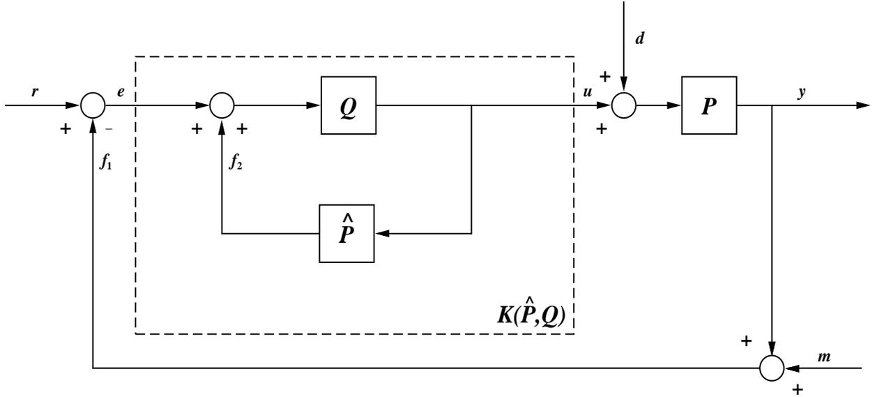
Figure 2: The IMC controller  $K(\hat{P}, Q) = Q(1 - \hat{P}Q)^{-1}$ .
