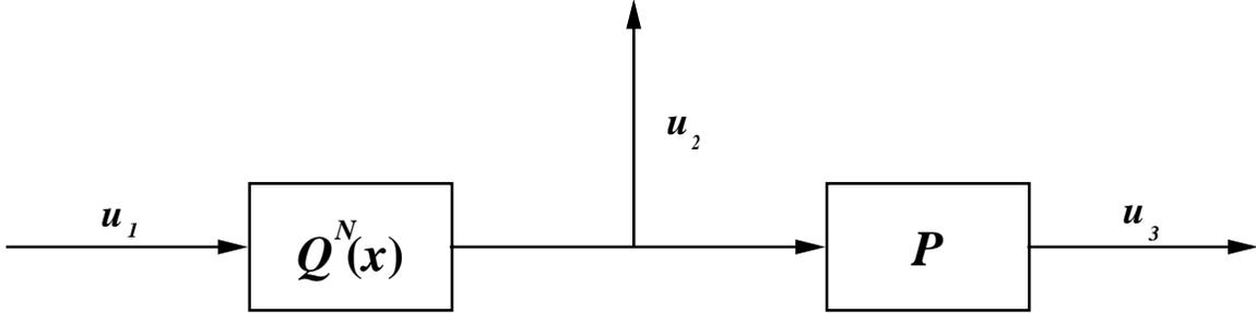
Figure 3: Open-loop system used to evaluate performance functionals and their subgradients using measurements.
