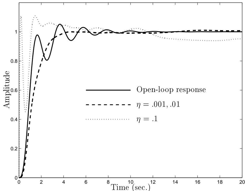
Figure 4: The output closed-loop step response of the tuned system for three levels of noise and the open-loop step response of the plant. The responses for  $\eta$  equal to .01 and .001 are indistinguishable.
