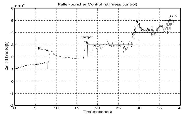
Figure 10. Controlled Force Application using Stiffness Feedback
