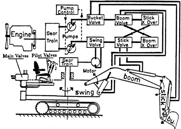
Figure 3. Excavator Hydraulics Circuit
