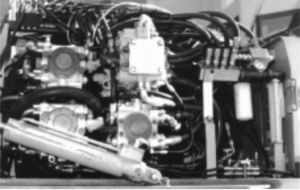
Figure 5. Hydrostatic Drive System
