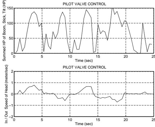
Figure 8. Machine Power and Head Speed with Valve Control
