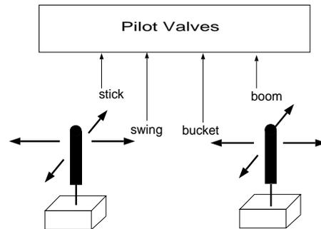
Figure 1. Standard Hand Controls
