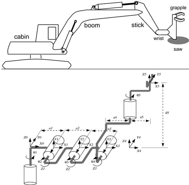
Figure 2. Feller-Buncher Schematic and Kinematic Configuration
