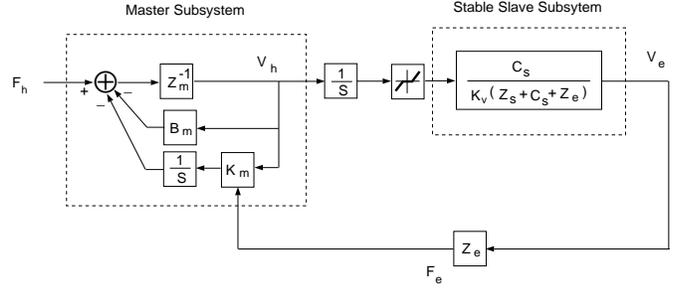
Figure 6. Schematic Diagram of Rate Control with Stiffness Feedback
