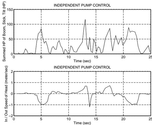
Figure 9. Machine Power and Head Speed with Pump Control
