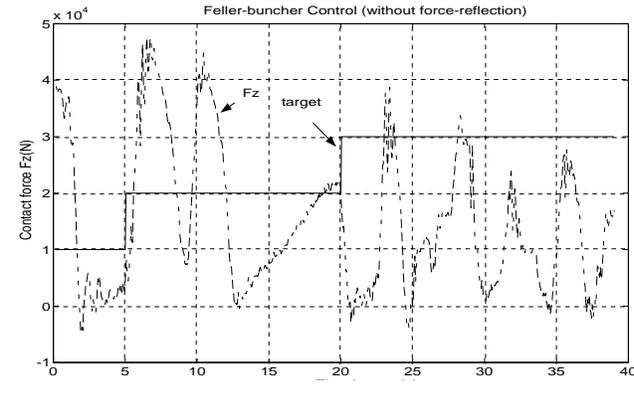
Figure 11. Attempts at Controlled Force Application without Force Feedback
