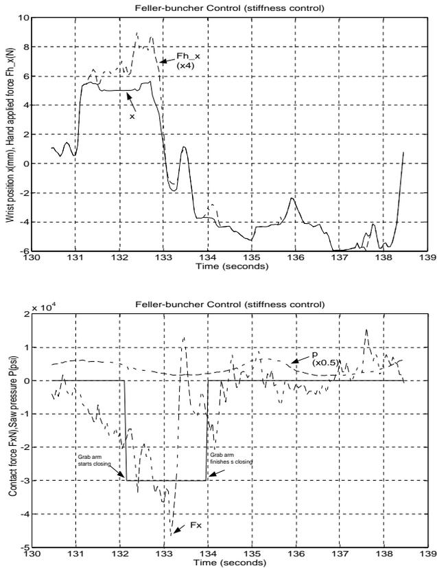
Figure 12. Hand-Controller and Feller-Buncher Radial Displacements and Forces During Tree-Cutting Process
