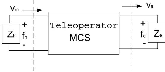
Figure 4 Two-port representation of a bilateral teleoperation system
