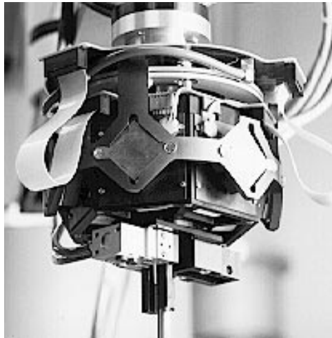
Figure 4: Fine Motion Robot Wrist using Lorentz Levitation: the flotor moves in six degrees of freedom over \sim \pm 5 mm in translation and \sim \pm 5^\circ in rotation.
