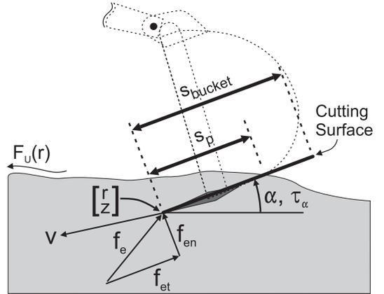
Figure 4: The Cutting Edge Frame and Dimensions.
