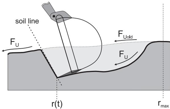
Figure 6: Ground Surface Dimensions are Updated and Stored in  $F_u(r)$ .
