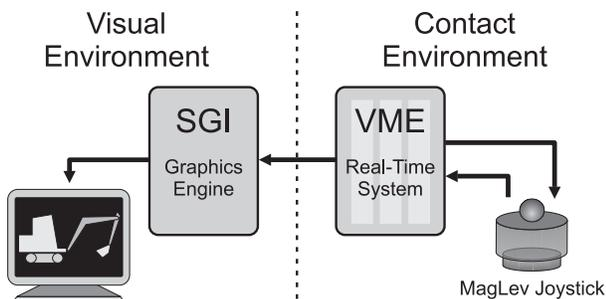
Figure 1: Excavation Simulator System.
