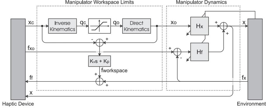
Figure 2: System Signal Flow and Control Between Master and Slave Sub-Systems.
