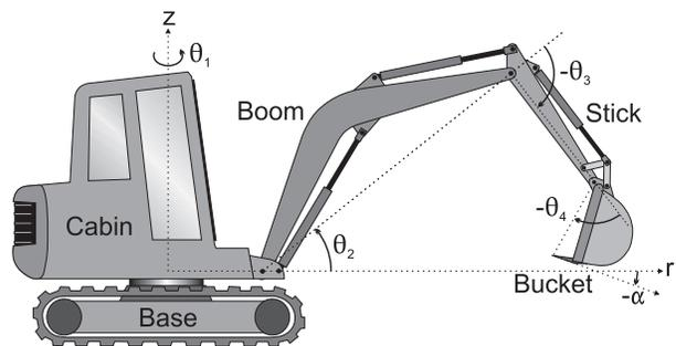
Figure 3: The Mini-Excavator, its Components and Coordinate Frames. For Bucket Details, see Figure 4.
