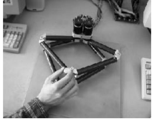
Figure 3: The Twin-Pantograph Haptic Mouse
