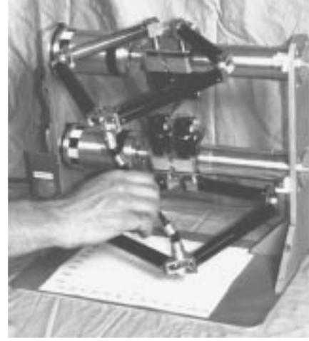
Figure 5: The Twin-Pantograph Haptic Pen
