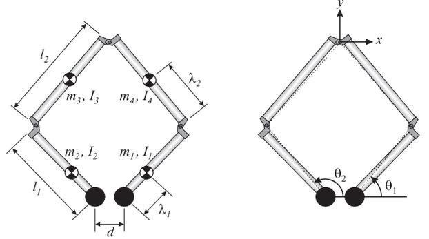
Figure 3: Pantograph configuration and parameters.
