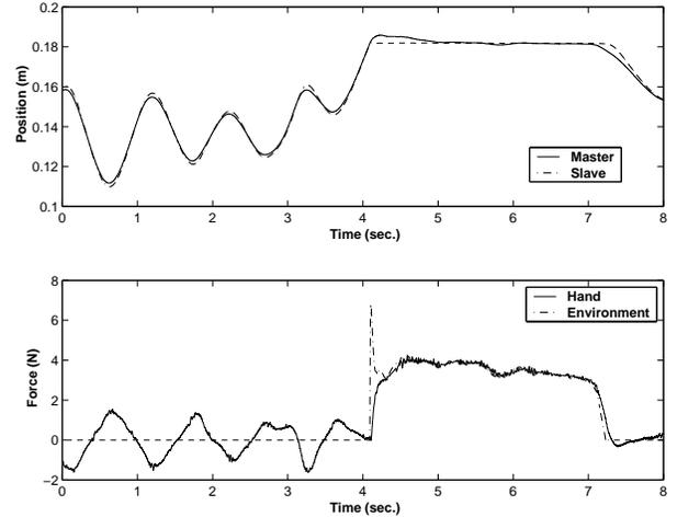
Figure 9: Four-channel with adaptive damping, tracking results.
