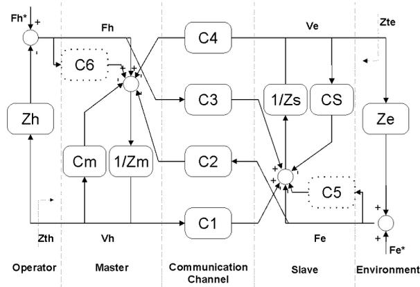
Figure 6: Four-channel architecture with local force feedback.
