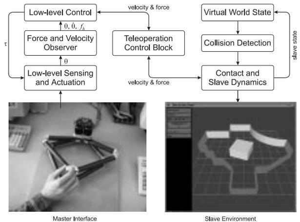
Figure 1: The virtual environment system architecture.
