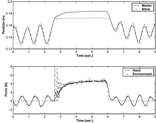
Figure 7: Two-channel position-force architecture, tracking results.
