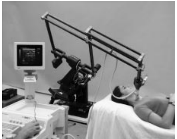
Figure 1: Experimental setup for robot-assisted ultrasound [1]. The 6-DOF parallel-linkage robot moves the ultrasound probe on the patient's neck for the carotid artery examination.
