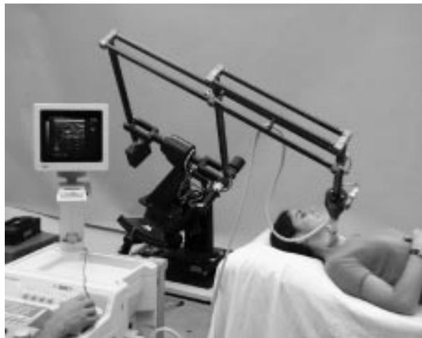
Figure 1: Experimental setup for robot-assisted ultrasound [1]. The 6-DOF parallel-linkage robot moves the ultrasound probe on the patient's neck for the carotid artery examination.
