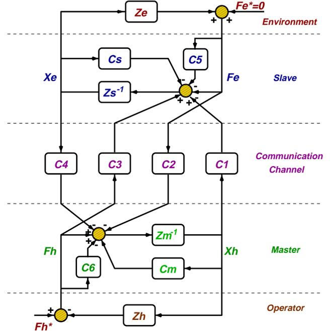
Figure 2. General block diagram of a four-channel teleoperation control system after Lawrence (1992), (Hashtrudi-Zaad and Salcudean, 1999).
