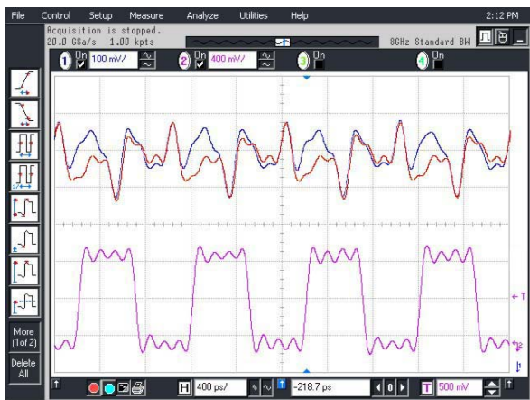
Fig. 10. Superimposed waveforms of a test chip on a 1GHz clock.
