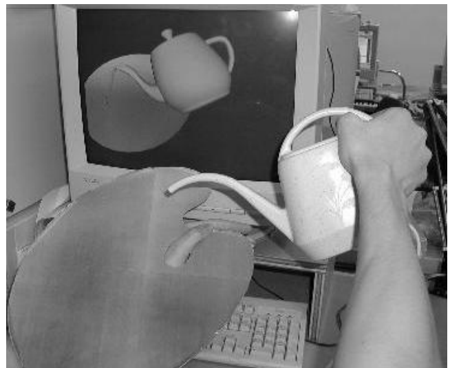
Figure 1: MetaMuse in use, showing props in front of rendered image. Note that the palette's surface has a colour pattern.
