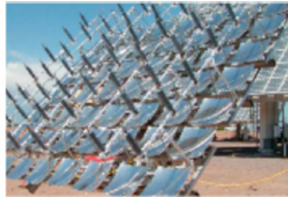
Microdishes can be passively cooled
