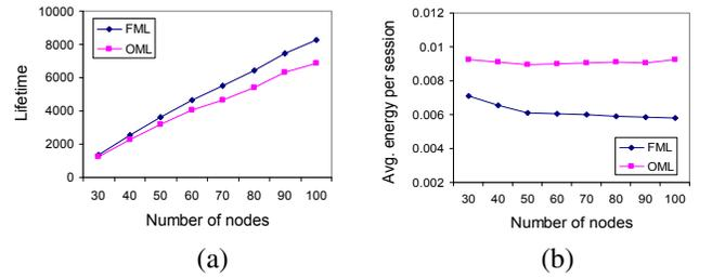
Fig. 8. A comparison of FML and OML in terms of (a) network lifetime and (b) average energy consumption per session for varying node density  $n$  in case of  $r_t = 9$ .
