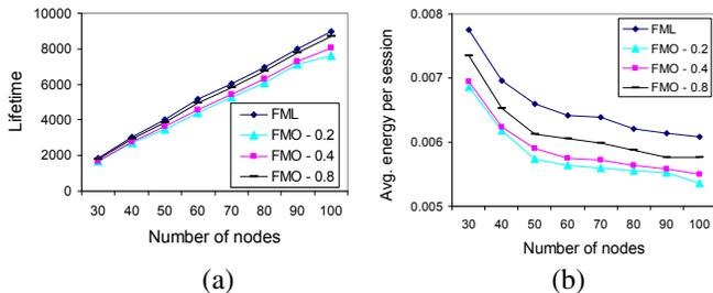
Fig. 10. (a) Lifetime and (b) average energy consumption obtained from FMO using various values for the parameter  $\Delta$  for varying node density  $n$ .
