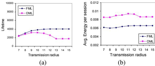
Fig. 6. A comparison of FML and OML in terms of (a) network lifetime and (b) average energy consumption for varying transmission radius ( $r_t$ ).
