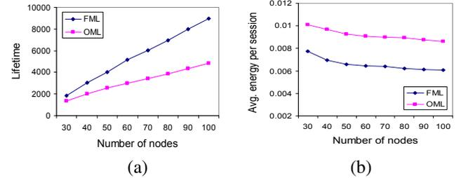
Fig. 7. A comparison of FML and OML in terms of (a) network lifetime and (b) average energy consumption per session for varying node density  $n$  in case of  $r_t = 12$ .
