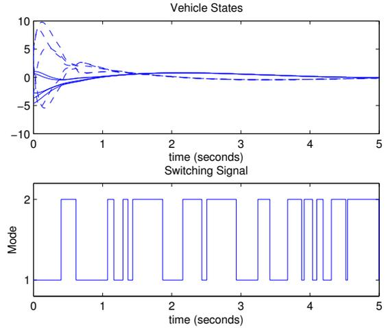
Fig. 2. Simulation results for the five vehicle system given by (3), (24) and Laplacian (25), with mode switches occurring according to the arbitrary switching signal  $\sigma$  shown in the bottom plot. By Corollary 1, GUAS under arbitrary switching for (3) was proven by showing GUAS under arbitrary switching for each block diagonal subsystem (7). Shown are the position (top plot, solid) and velocity (top plot, dashed) variables of each of the vehicles.
