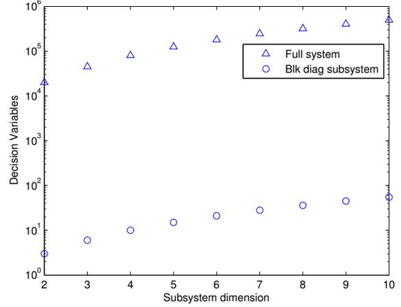
Fig. 1. Decision variables required in Matlab to solve an LMI to prove GUAS under arbitrary switching for a) a two mode distributed system with 100 subsystems ( $\Delta$ ) of total dimension  $100n$ , and b) a single block diagonal two mode subsystem ( $\circ$ ) of dimension  $n$ , for  $n \in \{2, \dots, 10\}$ .
