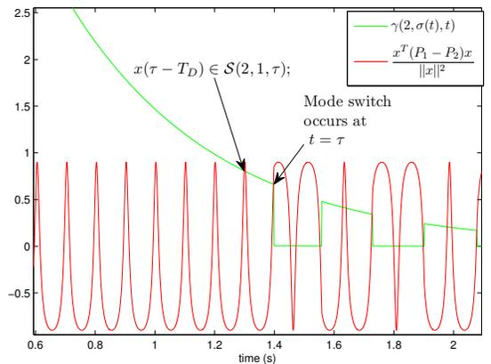
Fig. 5. From Figure 4, a close view of when  $x(\tau - T_D) \in \mathcal{S}(1, 2, \tau)$  for the first time at  $t = \tau$ . Clearly,  $V_{12}(\tau) > 0$ , satisfying the stability requirements imposed by Theorem 2.
