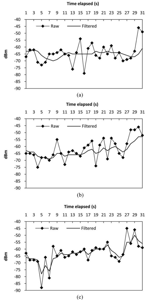
Fig. 7. Performance of RSSI filters implemented at the APs. (a) Moving average with ten sampled values. (b) Discrete Kalman ( $Q = 0.5$  and  $R = 5$ ). (c) Exponential smoothing ( $\alpha = 0.5$ ). Subject's speed is 1.0 m/s.
