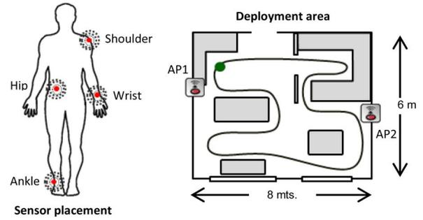
Fig. 5. Illustration of: 1) the WBASN devices' placement on a test subject for our experiments; 2) the trajectory followed by the subject during tests; 3) the deployment area with shadowed obstacles; and 4) the location of the AP. The dot indicates the starting and turn-around point.
