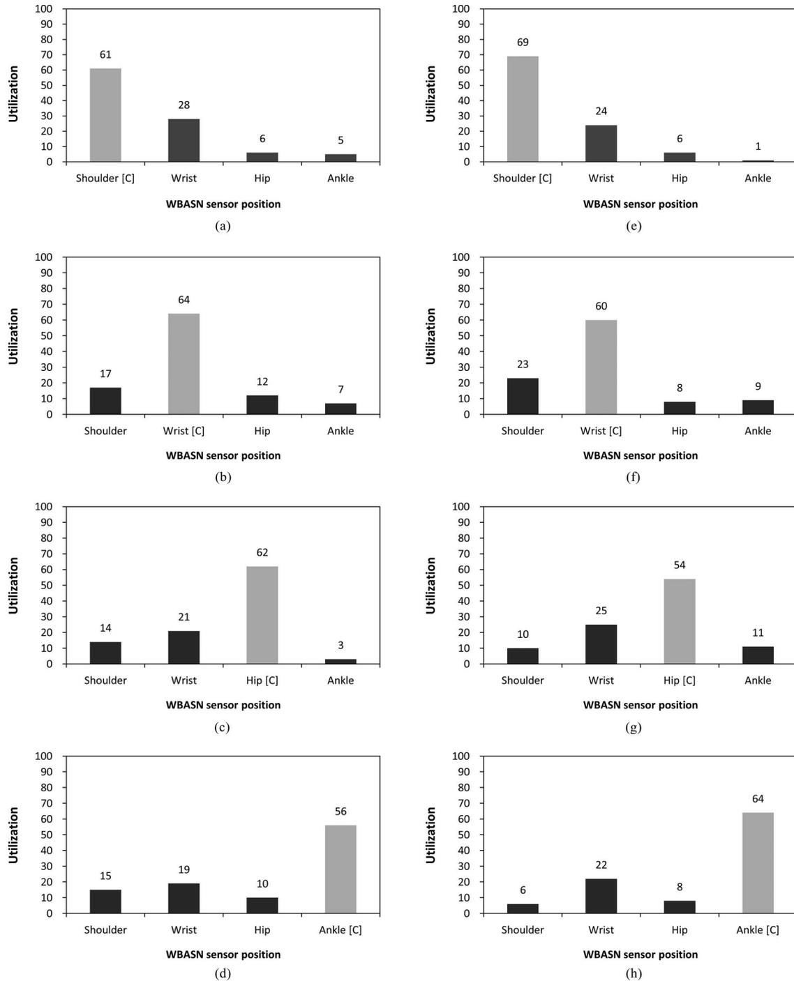
Fig. 9. Relay utilization for patients walking at 0.5 m/s as depicted in (a)–(d), and at 1.0 m/s as depicted in (e)–(h) for each respective sensor and the corresponding coordinator position [C].
