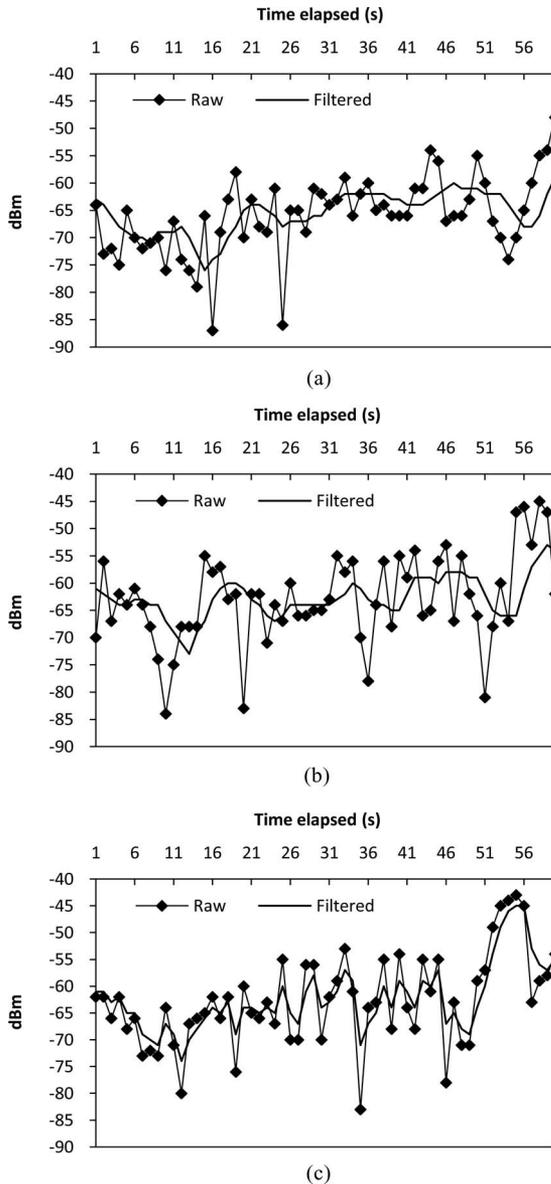
Fig. 6. Performance of RSSI filters implemented at the APs. (a) Moving average with ten sampled values. (b) Discrete Kalman ( $Q = 0.5$  and  $R = 5$ ). (c) Exponential smoothing ( $\alpha = 0.5$ ). Subject's speed is 0.5 m/s.
