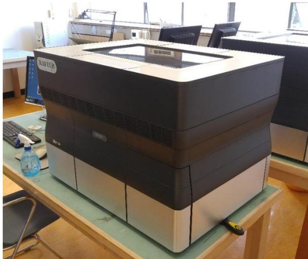
These two 3D printing technologies are fundamentally different and as such, they are both different in terms of material used, cost, functionality, etc. The Tinkerine DITTO PRO 3D printer has a lower absolute resolution, is much cheaper (both the cost of the printer and the build material), and can print parts much quicker. The Objet printers are able to achieve much higher precision and resolution, but cost considerably more and are also much slower in printing parts.
